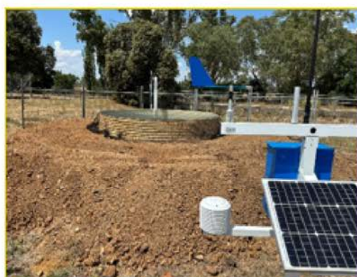
Figure 7: Tamworth brine evaporation experiment providing data for 50-year fill-evaporation cycle modelling
